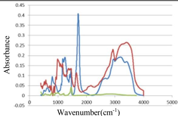
**Figure 3. The ATR spectrum of nanofiber of pure polyacrylic acid (blue), pure starch (red) and nanofiber of polyacrylic acid/starch (70:30)**
