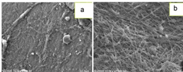
**Figure 2. Enzyme immobilization on the nanofiber polymer with stable conditions of parameters of electro spinning (a) Without plasma modification (b) with plasma modification**
