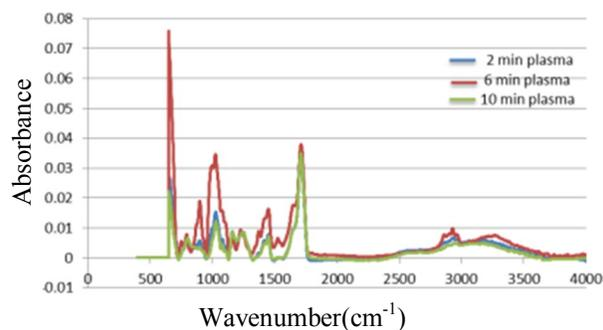
**Figure 4. FTIR spectrum of nanofiber with plasma modification**
