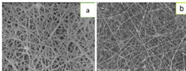
**Figure 1. The composite nanofiber with fixed parameter conditions of electro spinning procedure (a). Pure PAA (b). PAA/ starch (70:30)**
