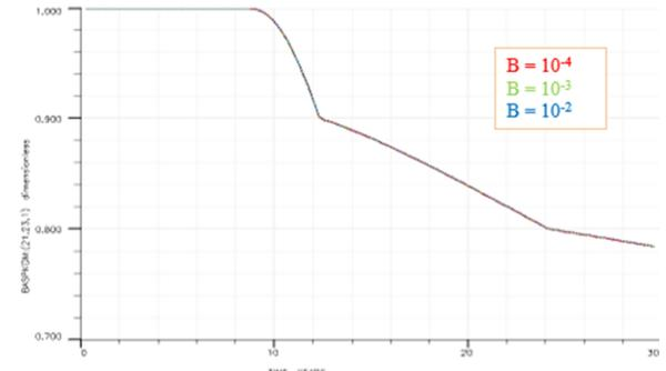
Figure 20. The effect of asphaltene plugging coefficient on the permeability damage
