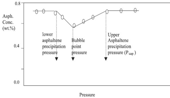
**Figure 1. The scheme of changing the procedure of asphaltene deposition on the basis of pressure decrease of reservoir (14)**
