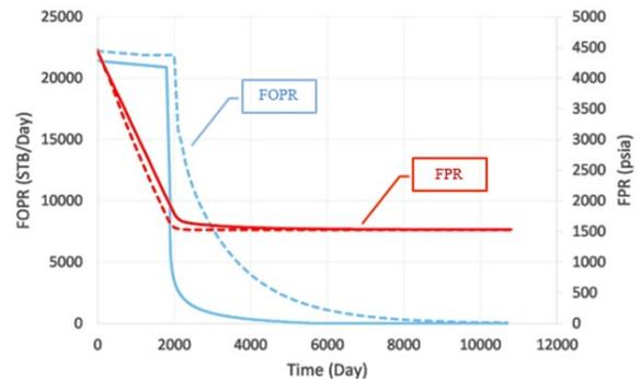
Figure 12. The flow rate of the produced oil, the process of pressure reduction and the effect of asphaltene precipitation on the flow rate of the production and drop of the pressure in the storage (CMG)
