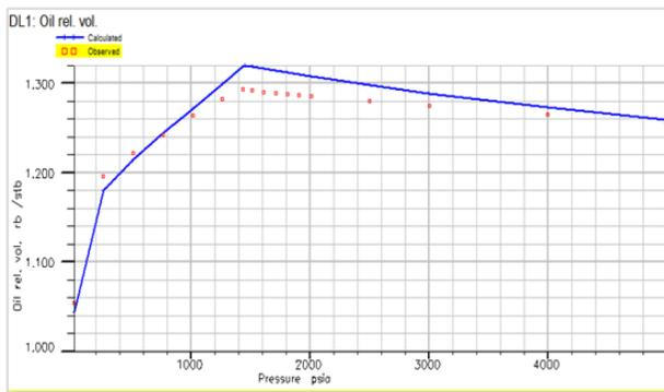
**Figure 3. Volume factor of formation in PVTi expansion test**
