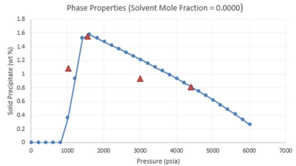
Figure 10. Asphaltene behaviour by pressure drop
