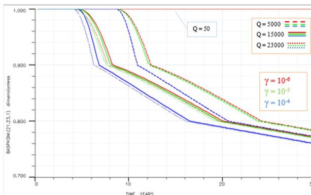
Figure 26. The effect of flow rate on entrainment coefficient and permeability damage
