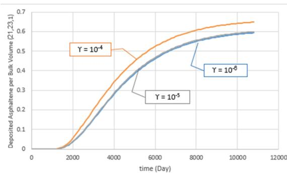
Figure 21. The effect of entrainment coefficient effect on asphaltene deposition
