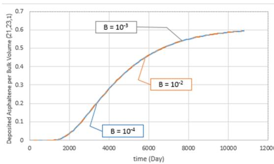
Figure 19. The effect of asphaltene plugging coefficient on the asphaltene deposition
