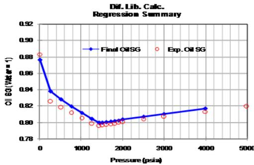
Figure 9. Determination of density of oil (Winprop)
