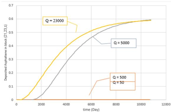
Figure 23. The effect of the different flow rates on asphaltene deposition
