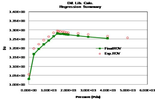
Figure 7. Determination of volume factor of the formation
