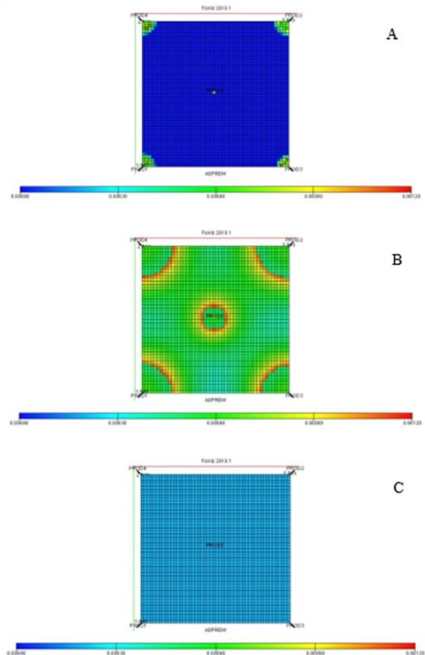
**Figure 16. A) Distribution of the asphaltene precipitation in the model at early stages of the simulation B) Distribution of the asphaltene at the middle time steps C) Precipitation distribution at the end of the stages.**
