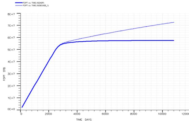
**Figure 15. The cumulative production of the oil and the effect of asphaltene precipitation on the cumulative production (E300)**
