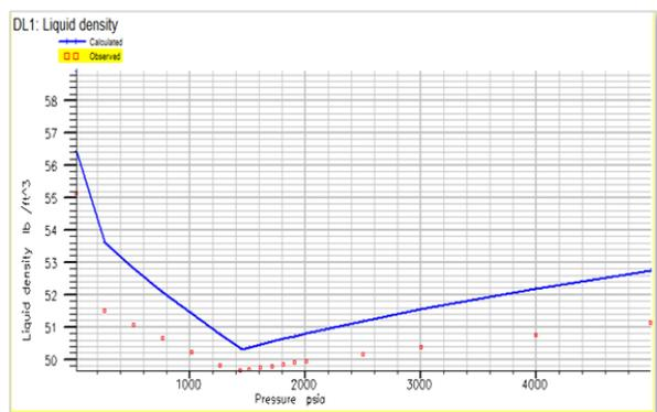
**Figure 4. Determination of fluid density (PVTi)**
