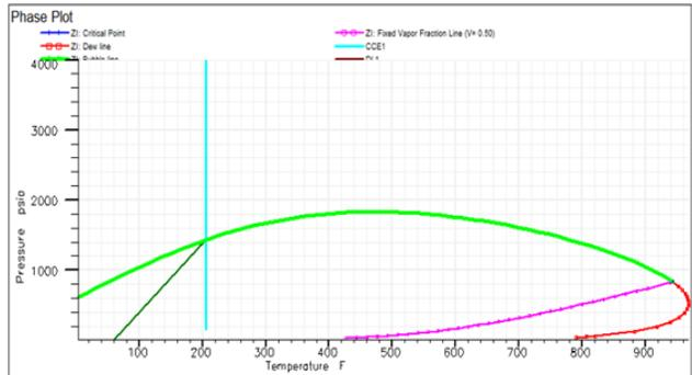
**Figure 2. Determination of fluid phase behaviour the oil. Molar percent of the asphaltene is calculated**
