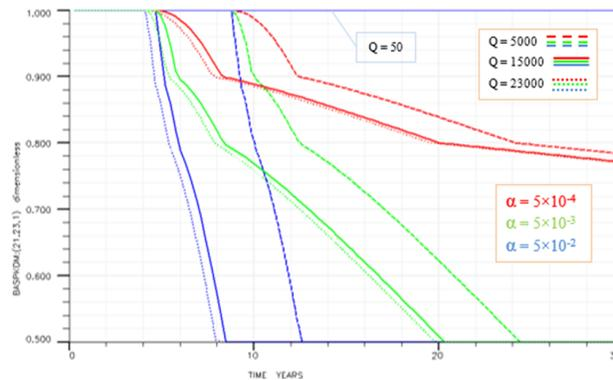
Figure 24. The effect of flow rate on the surface adsorption coefficient and permeability damage
