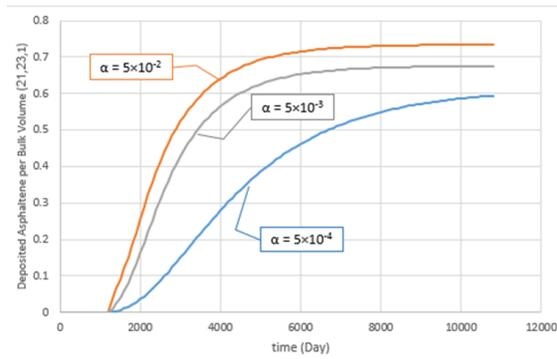
Figure 17. The effect of surface adsorption on the asphaltene deposition
