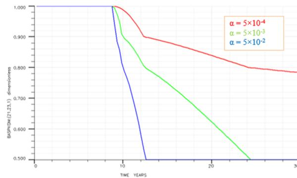
Figure 18. The effect of surface adsorption on the permeability damage.
