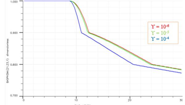
Figure 22. The effect of entrainment coefficient on permeability damage
