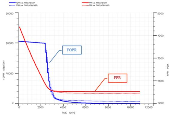
**Figure 13. The flow rate of the produced oil, the process of pressure reduction and the effect of asphaltene precipitation on the flow rate of the production and pressure drop in the storage (E300)**
