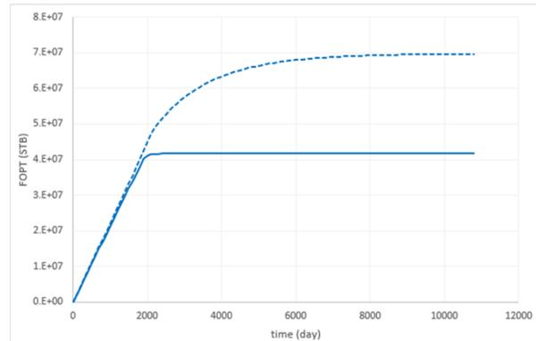
**Figure 14. The cumulative production of the oil and the effect of the asphaltene precipitation on the cumulative production (CMG)**
