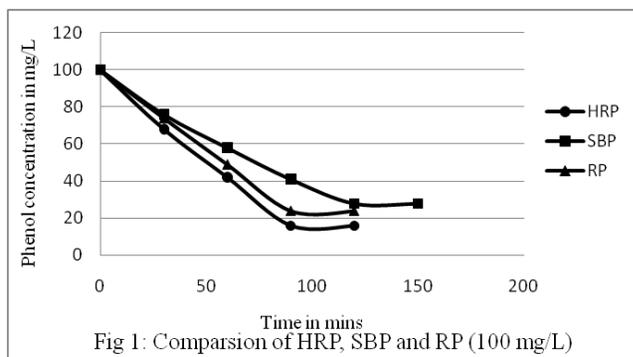
Fig 1: Comparison of HRP, SBP and RP (100 mg/L)
