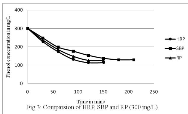
Fig 3: Comparison of HRP, SBP and RP (300 mg/L)
